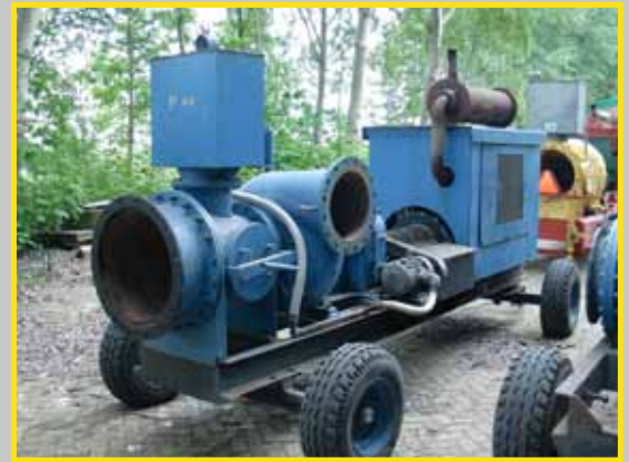
Capacity: 2500 M3/hour Engine: Scania D11. Pump: HK300
