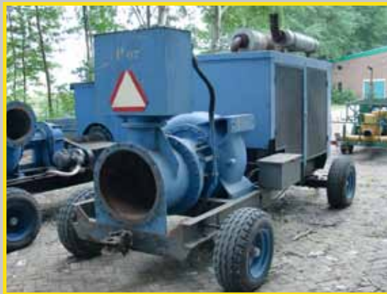
Capacity: 2500 M3/hour Engine: DAF 825. Pump: Nijhuis
