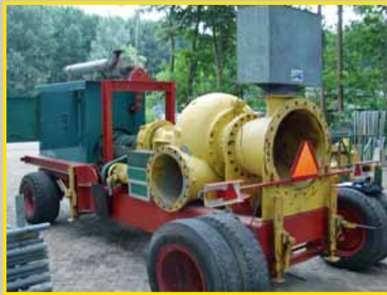
Capacity: 5000 m3/hour Engine: Scania D11 Engine. Pump: HK500
